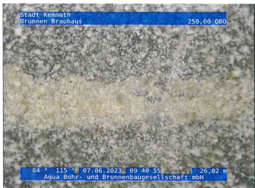
20, 00:20:33, 26.02m OK Filterrohr
